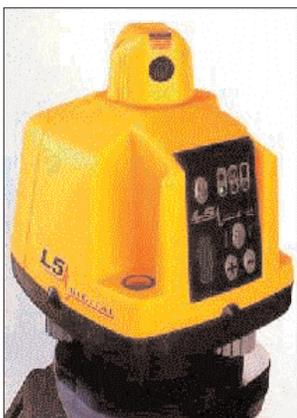
In its regulation for Non-Ionizing Radiation (29 CFR 1926.54), the Occupational Safety and Health Administration (OSHA) provides the standard for safe laser use. *All lasers used in construction are covered by this standard.* However, OSHA recognizes that the degree of hazard associated with low power lasers used in construction is relatively low and that Class 1 lasers are generally not hazardous.
